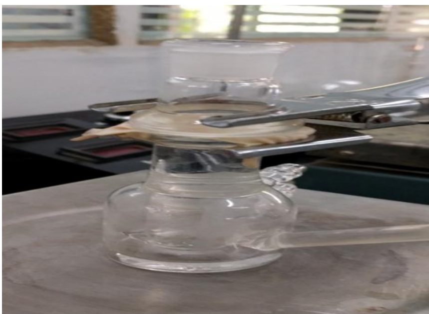
Fig. 4.2: Franz diffusion cell apparatus with mucosal membrane mounted between compartments.
