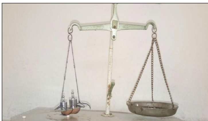
Fig 5: Determination of Bioadhesive strength by modified physical balance.
