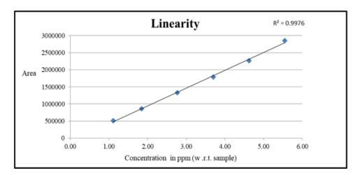
Figure 3: Linearity graph of O-Boc impurity.
