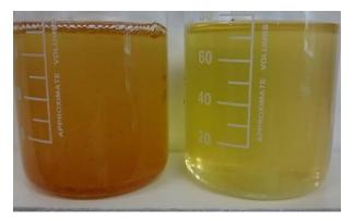
Fig 23: The purification of bio-ethanol using activated Carbon. The fig in the left is before purification and fig in the right is after purification.<sup>[6]</sup> The specific gravity of the ethanol changes from 0.85 to 0.81 ,which shows Removal of impurities from it.
