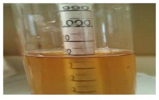
Fig 27: The specific gravity of the ethanol is observed by hydrometer and it is noted to be 0.85 at  $25^{\circ}$ C.
