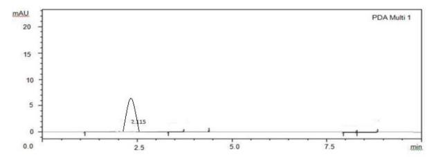
Fig. 6.35: Typical chromatogram for loq of fenoprofen.
