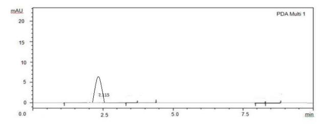
Fig. 6.35: Typical chromatogram for log of fenoprofen.
