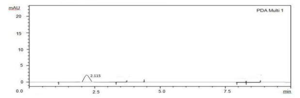
Fig. 6.34: Typical chromatogram for lod of fenoprofen.
