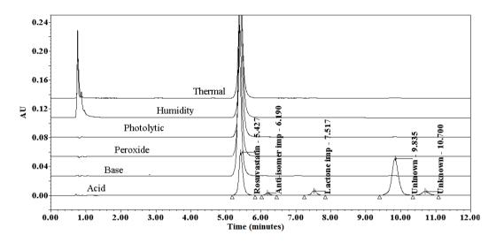
Fig. 2: Typical chromatograms of RSV forced degradation samples.
