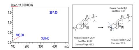
Figure 1: Full scan MS spectrum of  $\beta$ -sitosterol in APCI positive mode.
