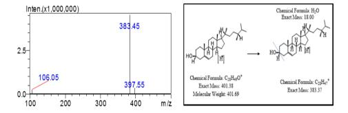
Figure 2: Full scan MS spectrum of campesterol in APCI positive mode.
