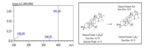
Figure 3: Full scan MS spectrum of stigmasterol in APCI positive mode.
