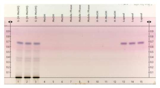
Fig. 5: HP-TLC chromatoplate for specificity after derivatization (540 nm).
