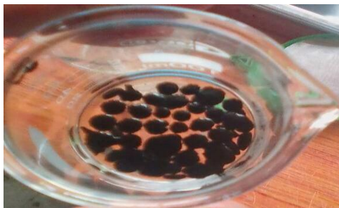
Fig. A: Photograph of the chitosan/magnetic cellulose/ sugarcane bagasse ternary bead.
