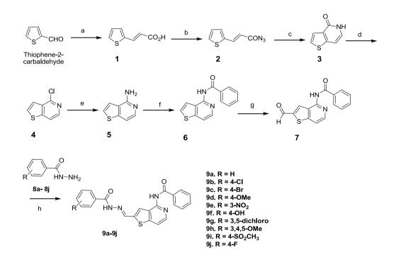
**Scheme 1:** *Experimental conditions:* a) Malonic acid, TBAB, water, microwave, 100°C, 5 min; b) Cyanuric chloride, N-methylmorpholine, NaN<sub>3</sub>, 0-5°C, 3h; c) Tributyl amine, diphenyl ether, 230°C, 30 min; (d) Trichloroisocyanuric acid, triphenylphosphine, toluene, reflux, 5.5 h; (e) aqueous; 28% ammonia, 1,4-dioxane, 150°C, 17 h; (f) Benzoic acid, HOBT, HBTU, DMF, rt,16 h (g) DMF, LDA, THF, - 78°C, 10 min (h) Benzohydrazides 8a-8j, ethanol, reflux, 30 min.
