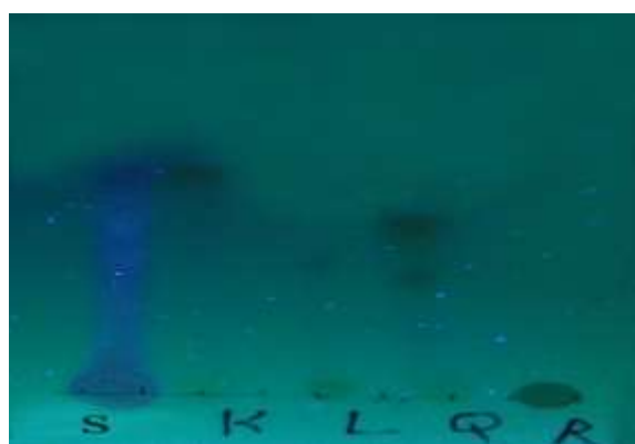
Figure (3-2): TLC chromatogram for the mobile phase A.vulgaris flavonoids extract (S), Quercetin (Q), Kaempferol (K), Luteoline (L) Rutin (R).
