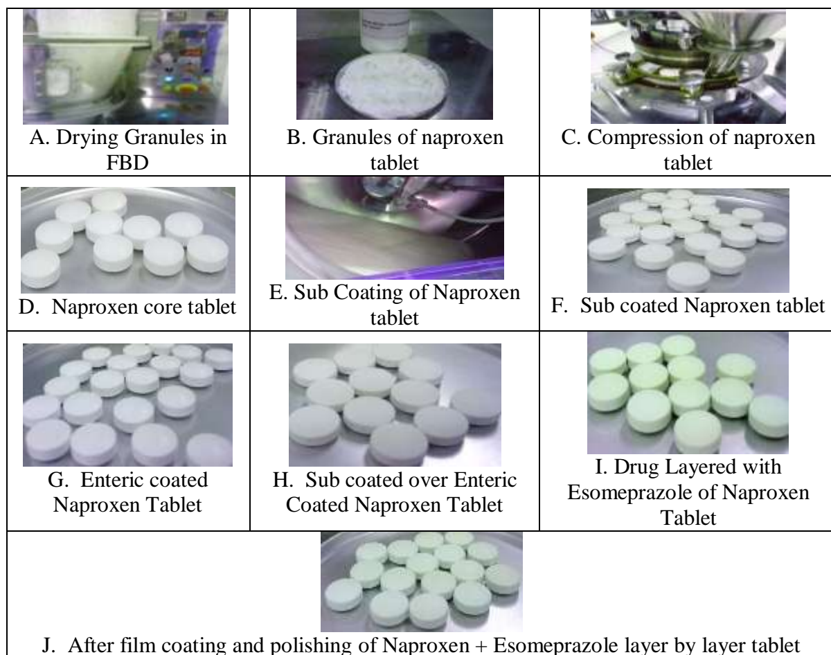
Figure 3 Pictorial presentations of steps of manufacturing of Naproxen and Esomeprazole layer by layer tablet
