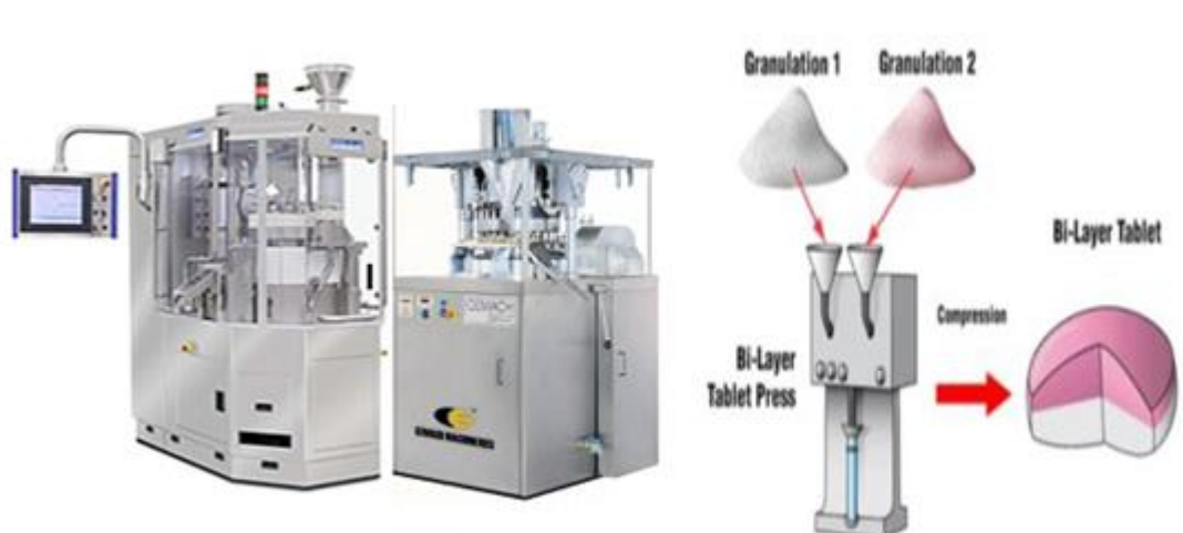
Fig.3 Double sided tablet press.
