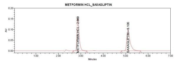
Fig:10 Photolytic Degradation Chromatogram for Metformin Hcl & Saxagliptin.
