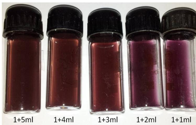
**Fig. 1 Visual colour change of gold nanoparticles at different concentrations of aqueous extract of *Alternanthera sessilis* with 1ml of gold chloride solution**
