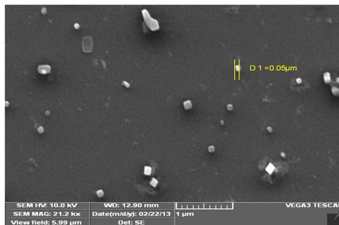
**Fig. 4 SEM micrograph of nanogold synthesized under sonication by *Alternanthera sessilis* extract**
