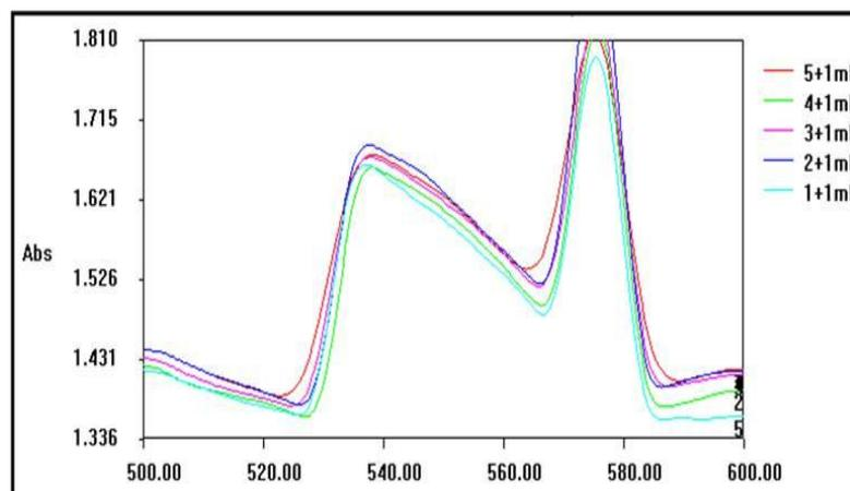
**Fig. 2** UV-visible spectra of synthesized nanogold using the aqueous extract of *Alternanthera sessilis*
