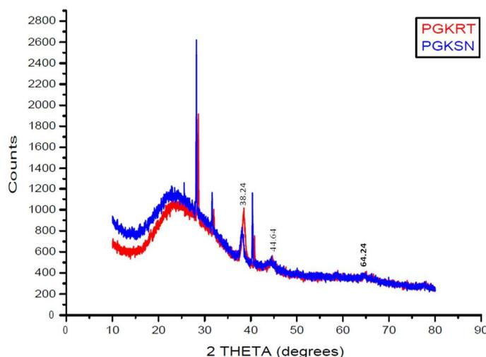
**Fig. 3** XRD patterns of synthesized nanogold using the aqueous extract of *Alternanthera sessilis* under room temperature (PGKRT) and sonication (PGKSN)
