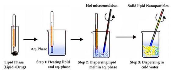
Figure 9: Micro-emulsion based method.<sup>[1]</sup>
