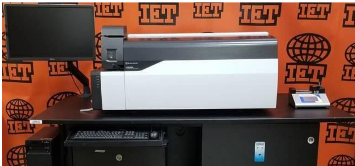
Fig: 8 Shimadzu LCMS-8050. Triple Quadrupole Liquid Chromatograph Mass Spectrometer (LC-MS/MS) (p/n 225-19610-44) complete with Edwards XDS46i vacuum pump (p/n A731-01-983), and Lab Solutions LCMS PC workstation with license.
