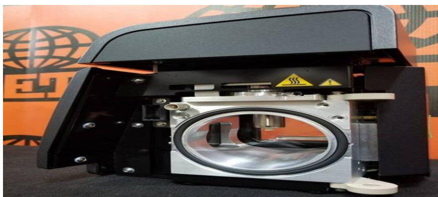
Fig:9 Shimadzu APCI probe (p/n 225-19601-58) for the LCMS-8050 Triple Quadrupole Liquid Chromatograph Mass Spectrometer (LC-MS/MS).
