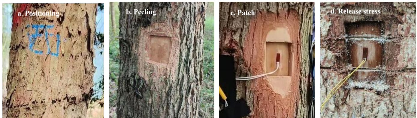
Figure 1. Growth strain measurement of Eucalyptus cloeziana ( E. cloeziana ).
