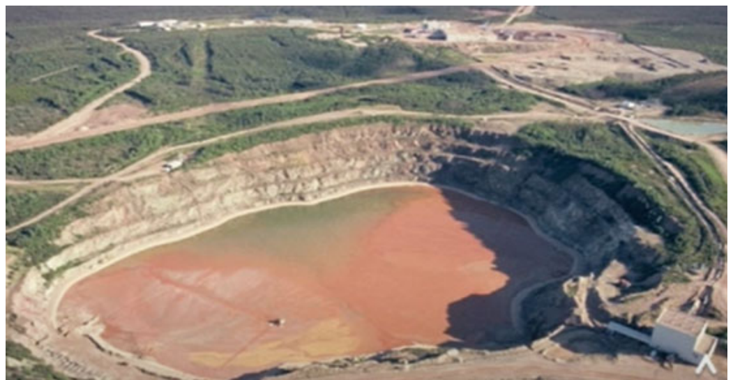
Figure 16. Rabbit Lake open-pit mine with tailings filling progress.
