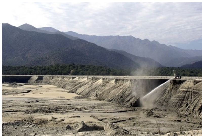
Figure 4. Mine tailings reprocessing at Los Colihues TSF using high-pressure water jets, El Teniente Copper Mine, Chile.
