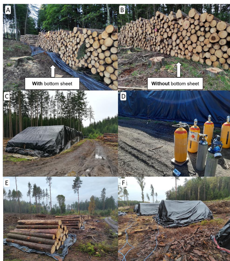
Figure 1. Visualization of EDN log stack fumigation under different (A–C) and identical (E,F) conditions. (A) Detail of the lower part of the log stack with bottom sheet; (B) detail of the lower part of the log stack without bottom sheet; (C) fumigated log stacks covered by an upper tarpaulin tent; (D) EDN application from the cylinder; (E) uncovered log stacks with bottom sheet; (F) fumigated covered log stacks with bottom sheet.
