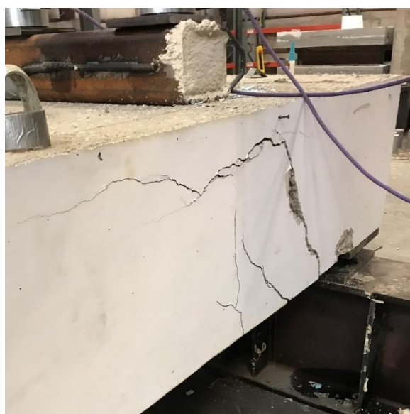
Figure 13. Failure mode when loaded at 1.25d .
