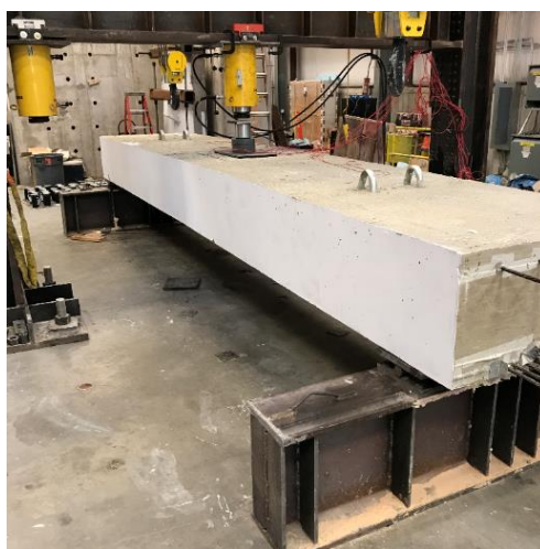
Figure 4. Midspan test setup and instrumentation: (a) test setup sketch and (b) test setup photo.
