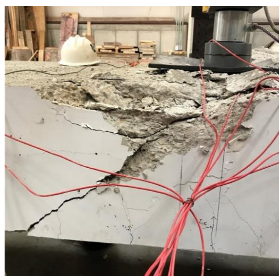
Figure 11. (a) Load–deflection relationship and (b) failure mode when loaded at midspan.
