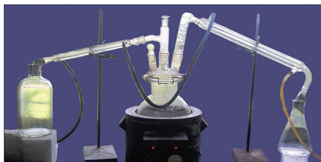
Figure 1: Mochikayantra (a distillery described in Sanskrit verse for the preparation of Vasarishta built upon Mritasanjeevani Sura )
