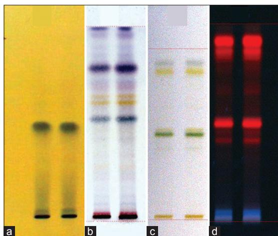
Figure 1: Graphical representation of phytochemical screening for the extracts/fractions. (a) Sprayed with ferric chloride solution at visible light; (b) sprayed with vanillin-sulfuric acid solution at visible light; (c) sprayed with p-anisidine-hydrochloride solution at visible light; (d) sprayed with aluminum trichloride solution at 366 nm
