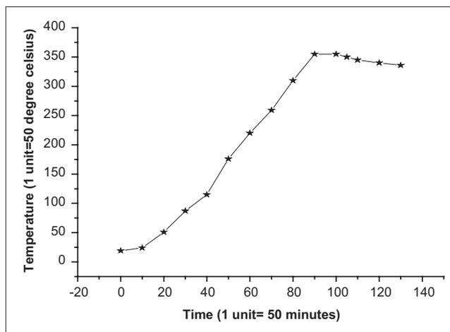
**Graph 2:Temperature pattern in electric muffle furnace during Putapaka process**
